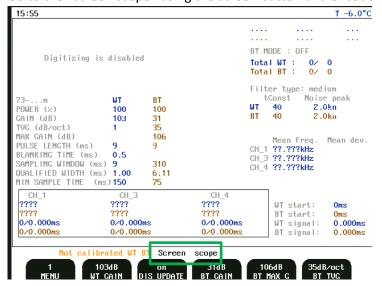
In MENU 3 make sure "SL RANGE" is set to 1-4m. The parameter "WT SAMPLE" is the ping length in shallow water 1-4m. Leave this at default 2ms.
